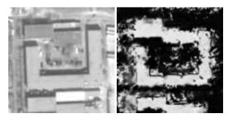
Figure 1: U-shaped building represented in a satellite image (left) and a DSM, which contrast has been enhanced by nonlinear clipping (right).
