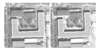
Figure 2: Matching without shape prior. Left: initial state close to the desired solution. Right: result without shape prior, "leak" of the active contour.
